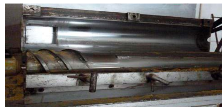
Figure 3.10.9 – Detail of the inner part of the hulling roller
