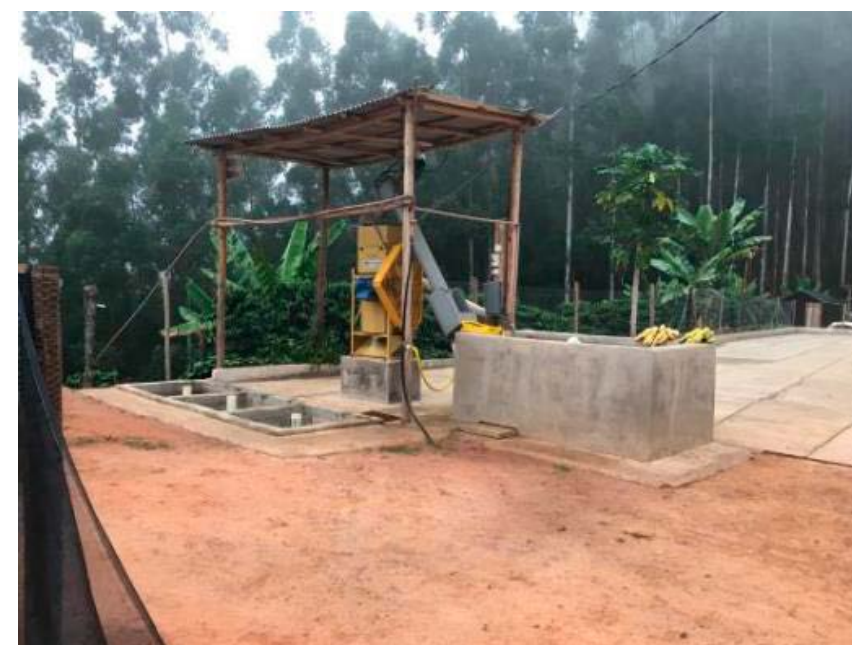
Figure 3.8.2: Processing Unit, consisting of a washing tank, a hulling machine/washer and SLAP. Sítio Conquista
