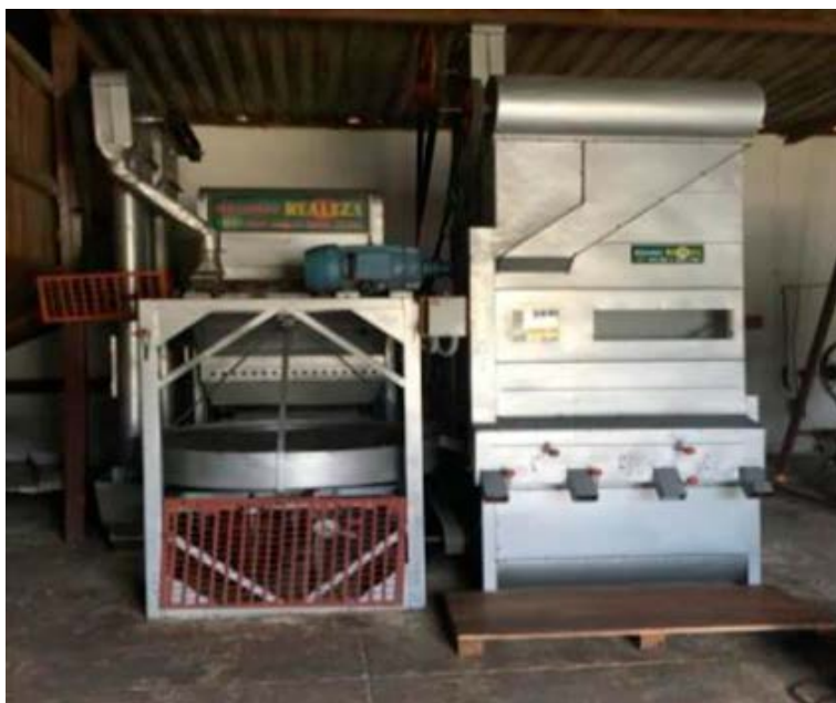
Figure 3.10.6 – Wet-process hulling roller and classification row
