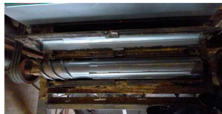
Figure 3.10.8 – Upper view of the hulling roller (open cover)
