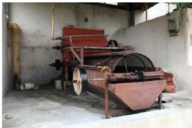
Figure 3.10.3 – Floater hulling machine developed by Mr. Cornélio
