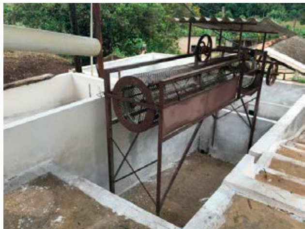
Figure 3.10.2 – Cylinder for separation of overripe floaters
